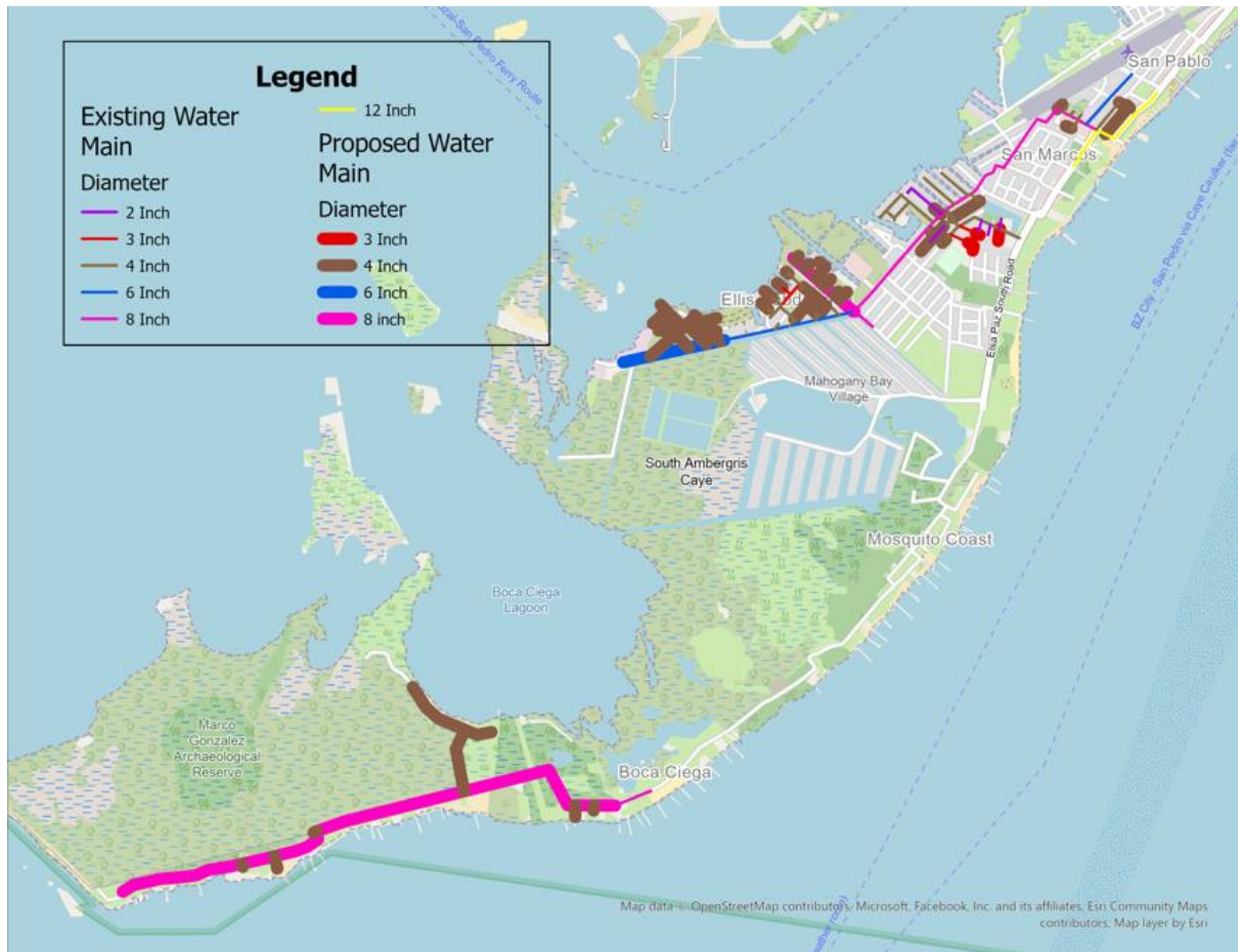
Figure 60 – Slide of Existing and proposed water Main, South San Pedro Water Network Expansion.
